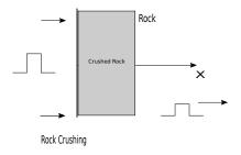
Note that the transmitted stress wave is reduced due to rock crushing.
