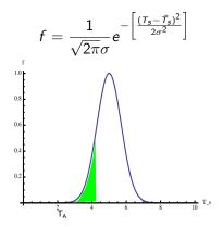
The green shading shows springs that have broken after the application of an individual spring tension  $T_s$ .
